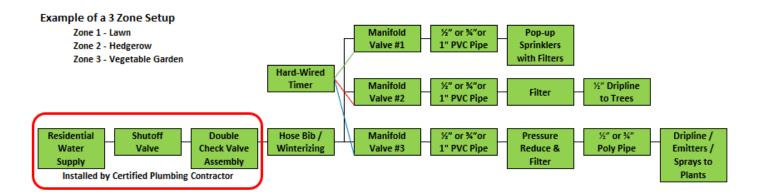
The tie-in to the main water supply (from the city meter to your home) includes a shutoff valve and double check valve assembly to prevent back flow. This **MUST** be done to municipal building code and will need to be installed by a certified plumber. Backflow prevention is legally required on **ALL** irrigation systems to prevent irrigation water and possible contaminants from siphoning back into your residential water system.
